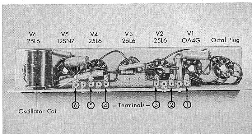
Figure 23. Bottom View of Electronic Chassis
