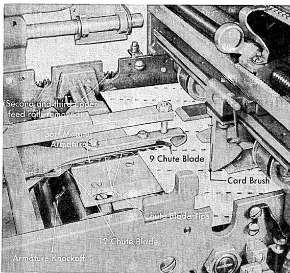
Figure 5. Sensing the Card
