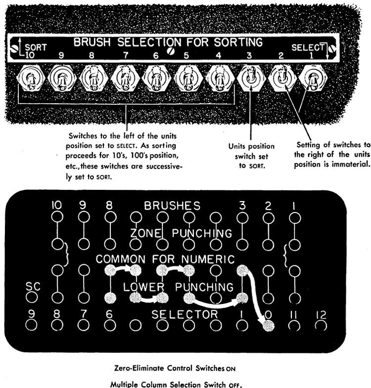
Figure 46. Control Panel Wiring - Zero Elimination
