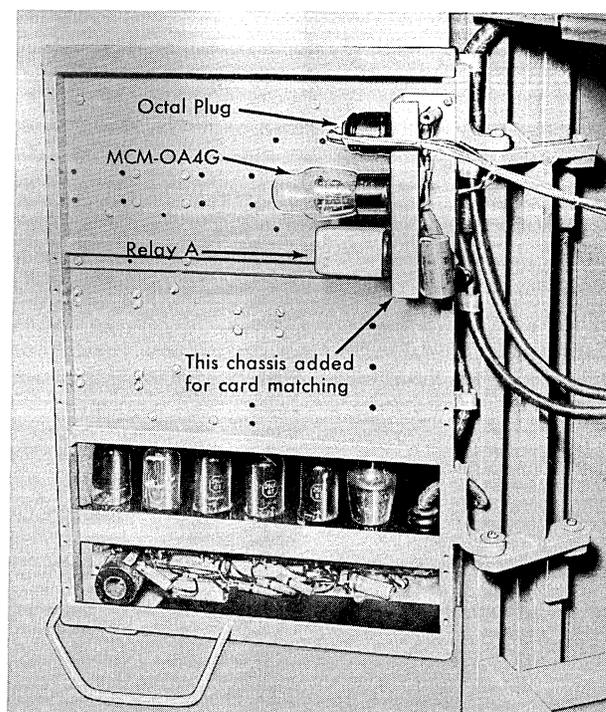
Figure 42. Card Matching Tube Chassis
