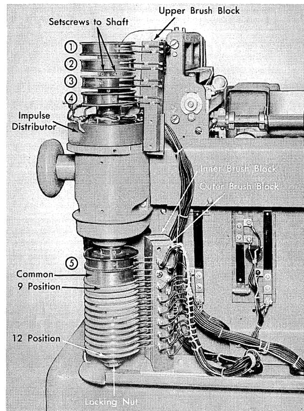
Figure 31. Counter Commutators and Impulse Distributor
