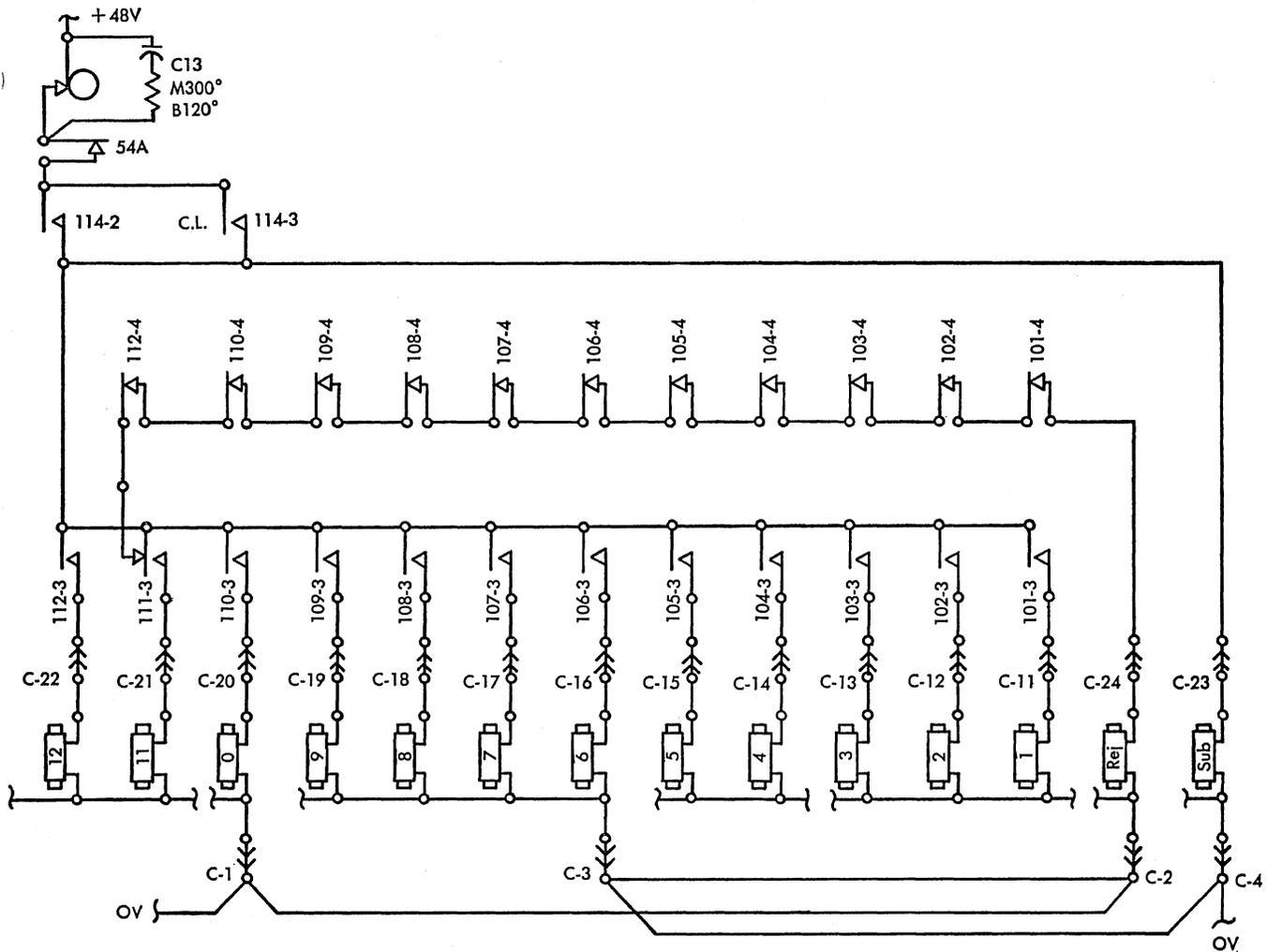
Figure 65. Counter Magnet Schematic
