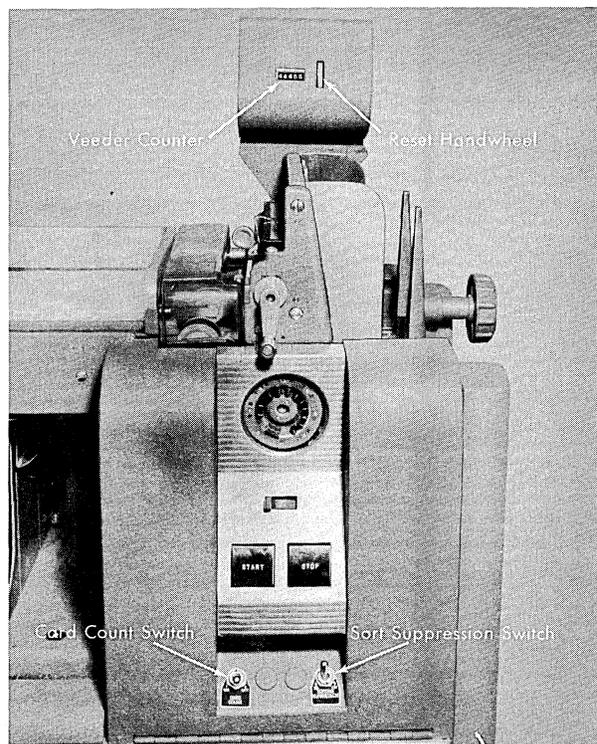
Figure 35. Auxiliary Card Counting Device
