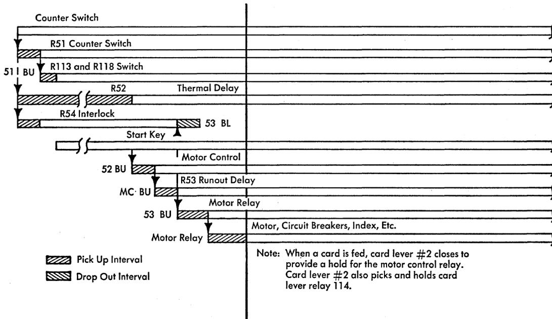
Figure 62. Conditioning Circuits (Sequence Chart)
