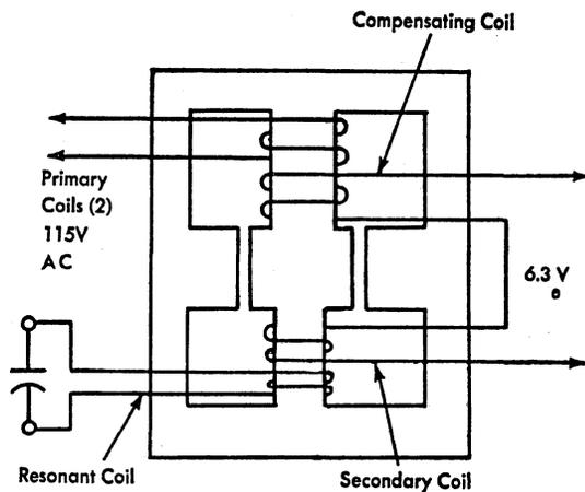
Figure 59. Schematic of Filament Voltage Transformer
