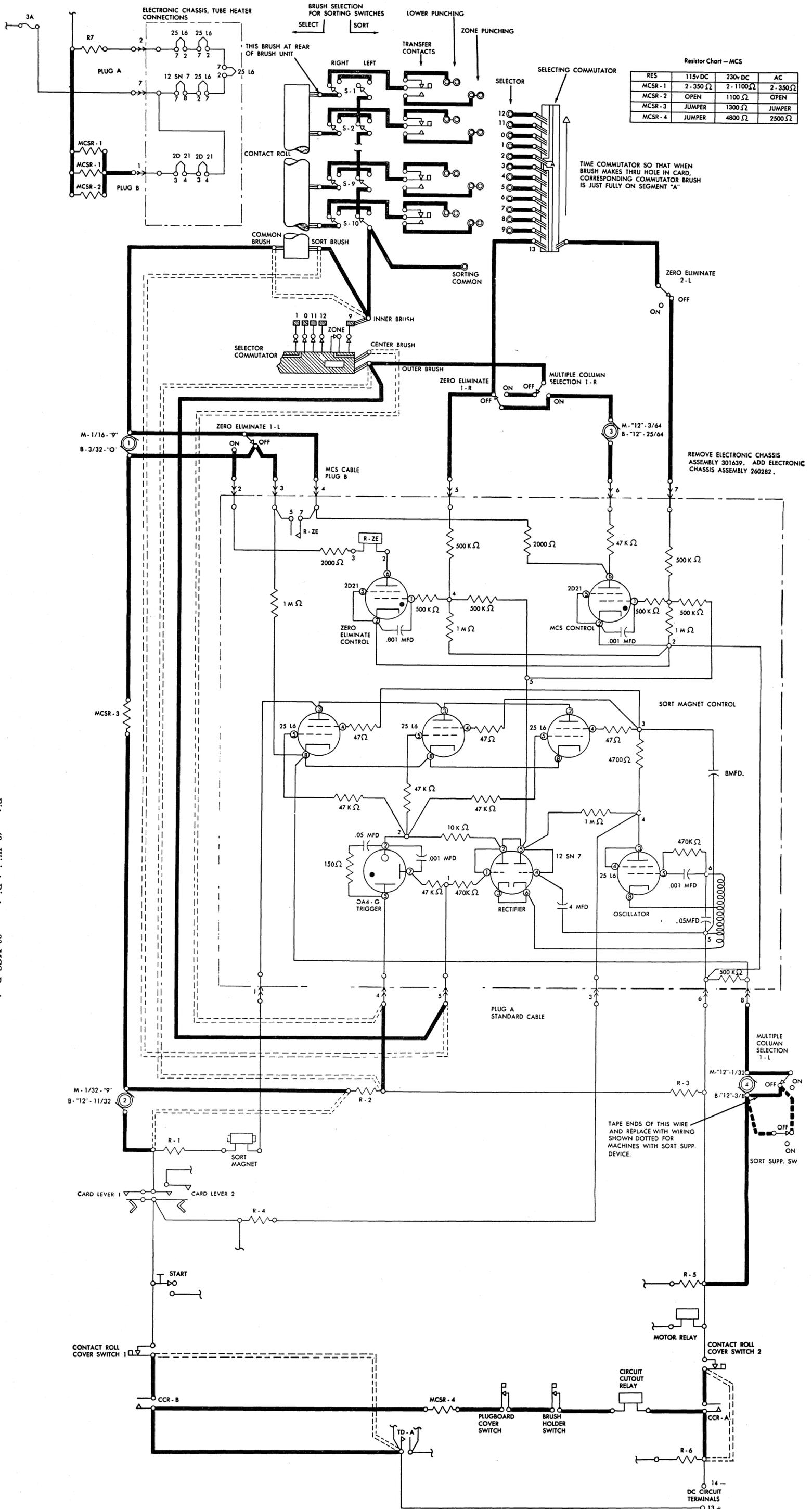
Figure 49. Wiring Diagram - 82 MCS Devices
