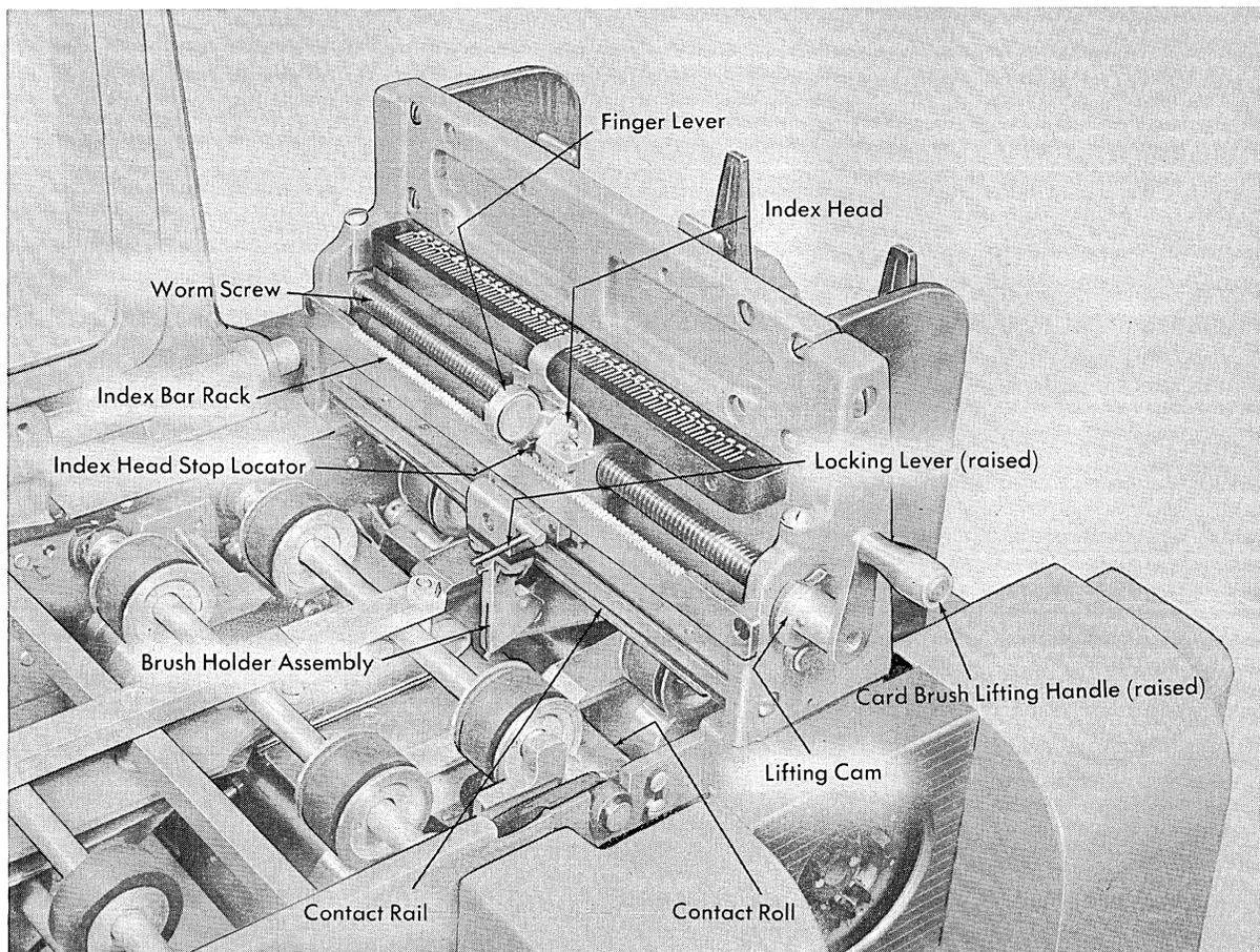
*Figure 9. Removing the Card Brush Assembly*
