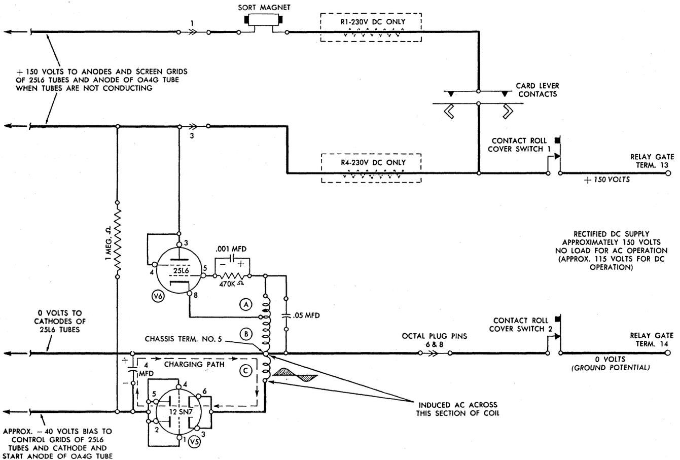
Figure 24. Schematic of Oscillator and Rectifier
