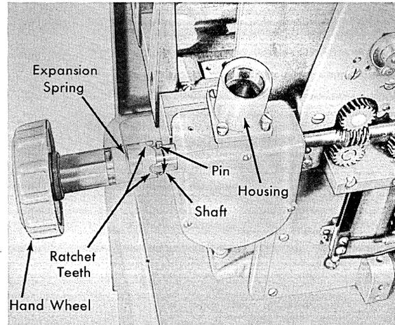
Figure 14. Declutching Hand Wheel
