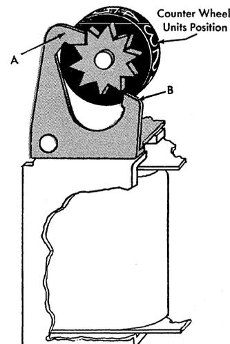
Figure 55. Counter Magnet Energized
