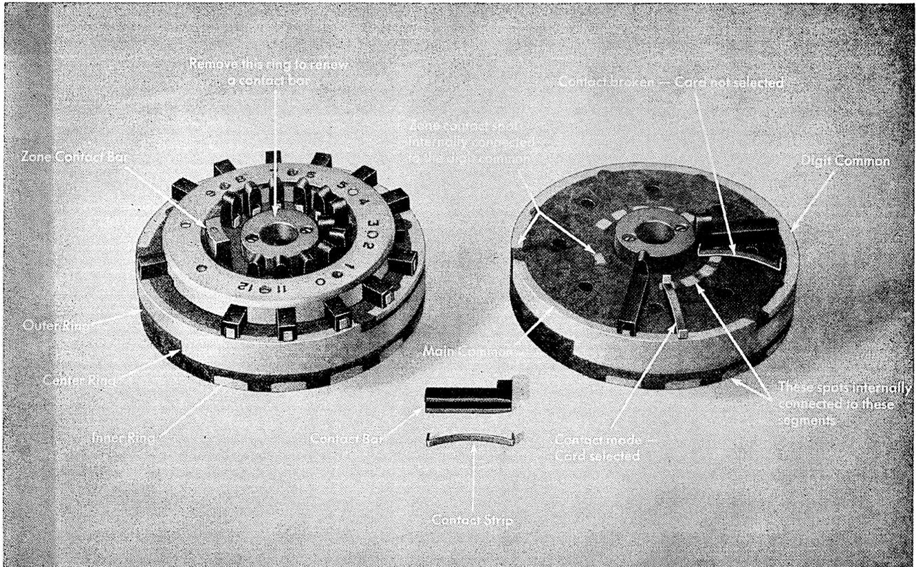
Figure 12. Commutator Assembly
