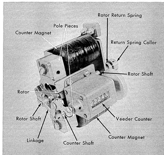
Figure 37. High Speed Card Counter Assembly
