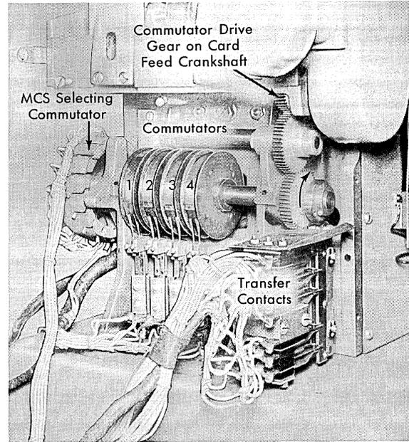
Figure 47. Internal Controls - MCS Device
