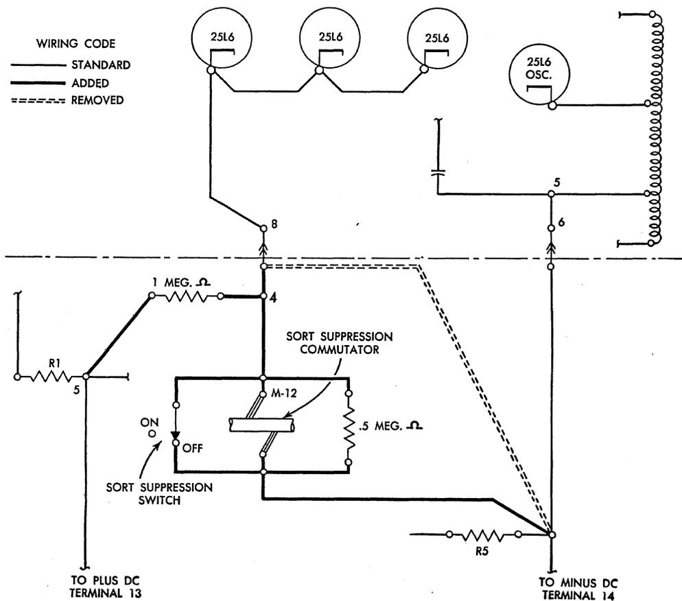
Figure 39. Wiring Diagram - Sort Suppression Device, Type 82
