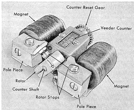
Figure 30. Type 75 Card Counter Assembly
