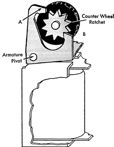
Figure 56. Counter Magnet Normal
