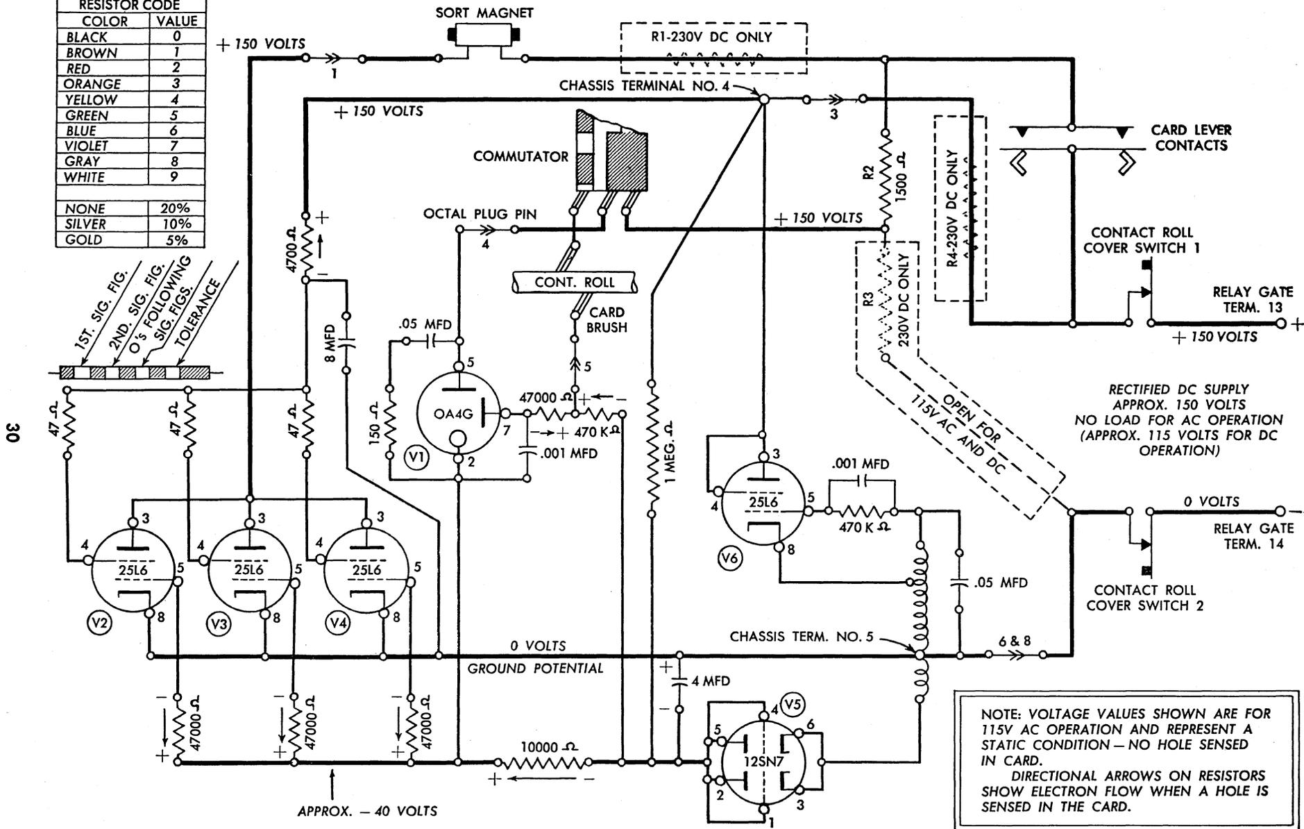
Figure 25. Schematic of Type 82 Sorting Circuits
