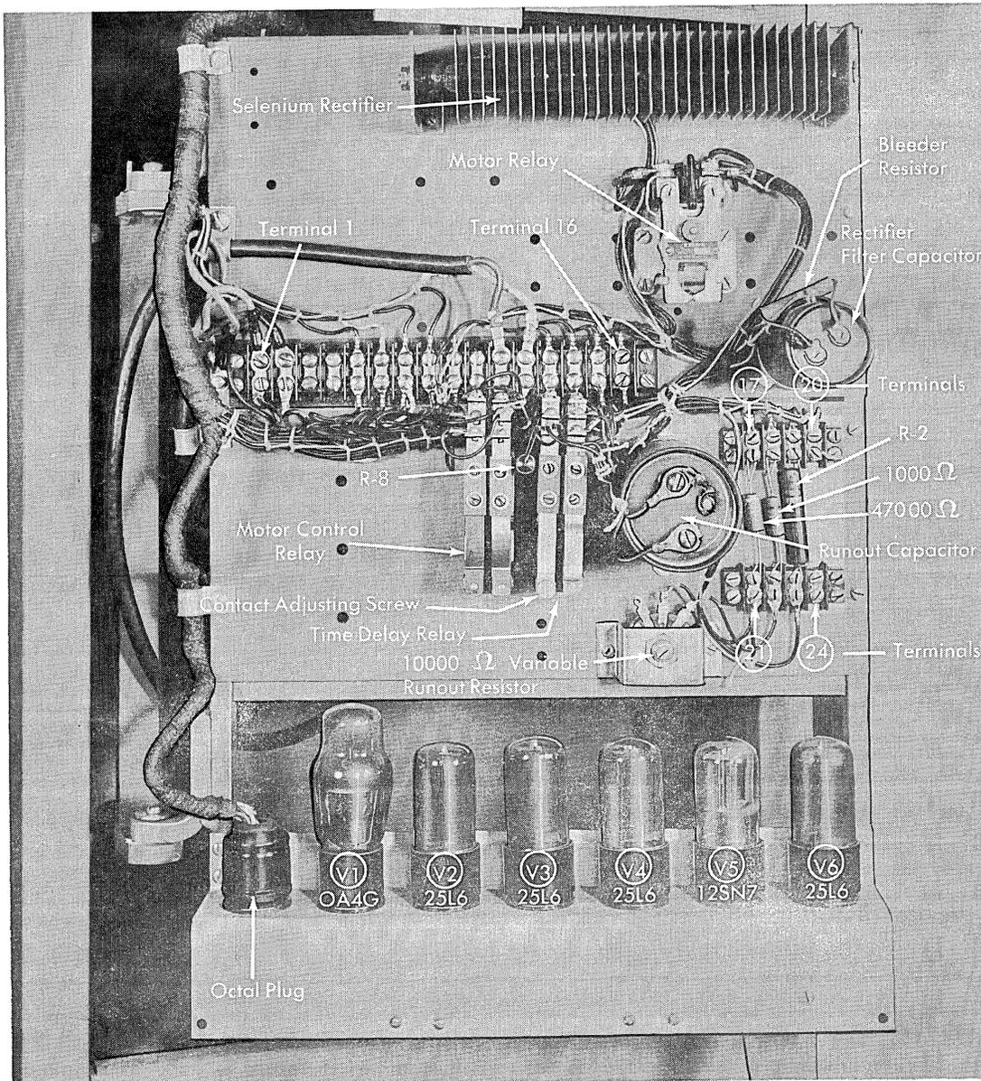
Figure 22. Relay Gate and Electronic Chassis
