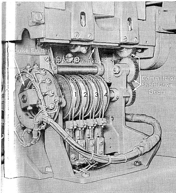
Figure 52. Internal Controls - Group Sorting Device
