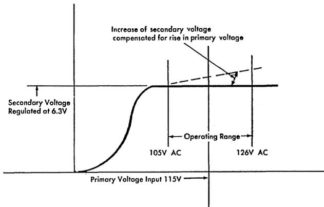
Figure 60. Schematic of Filament Transformer Output
