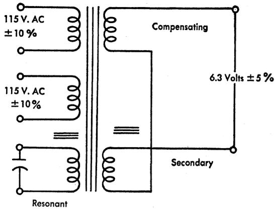
Figure 58. Filament Voltage Transformer (Schematic)
