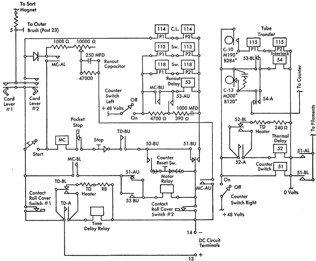
Figure 61. Start and Run Schematic
