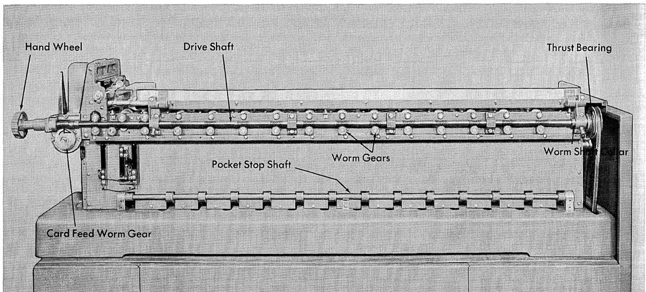
Figure 13. Main Drive Shaft and Pocket Stop Shaft
