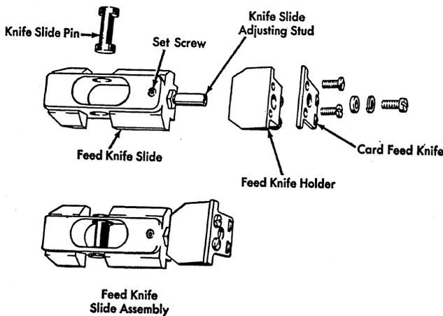
Figure 18. Feed Knife Slide Assembly
