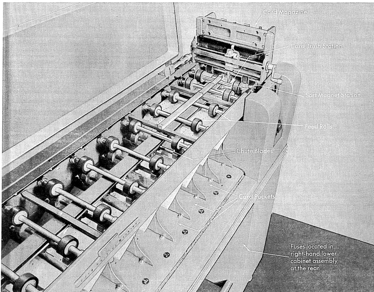
Figure 1. Card Transport Through the Machine
