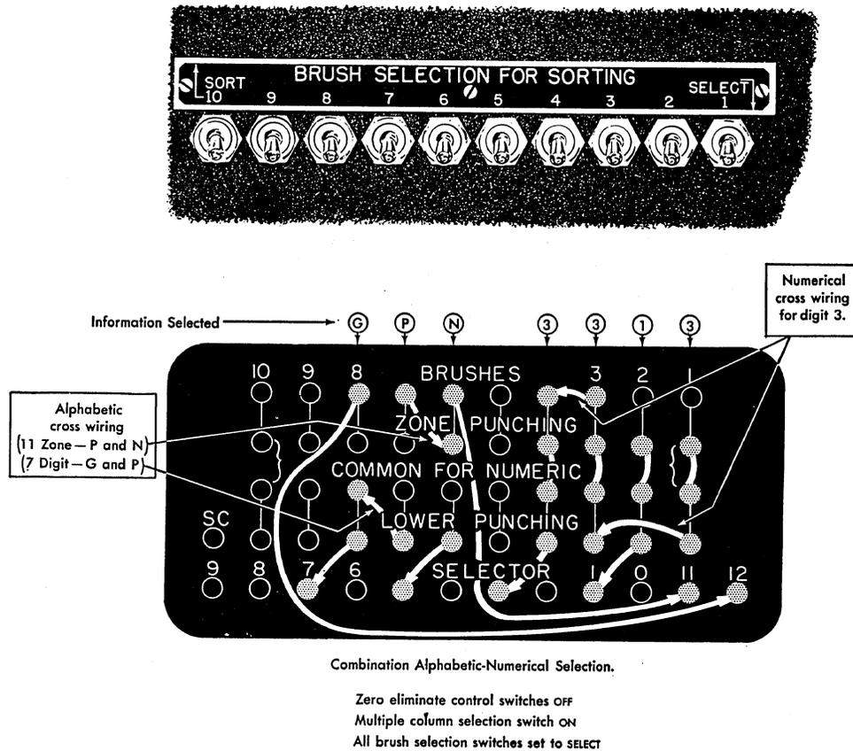
Figure 45. Control Panel Wiring - Multiple Column Selection
