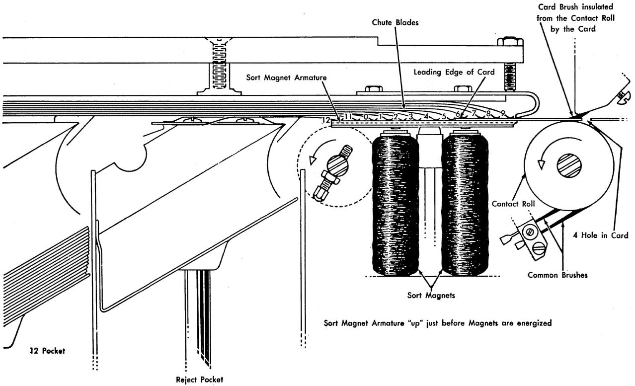
Figure 6. Position of Chute Blades Prior to Sort Magnet Energization
