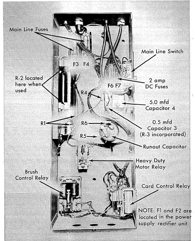
Figure 33. Type 75 Sorting Relay Cabinet
