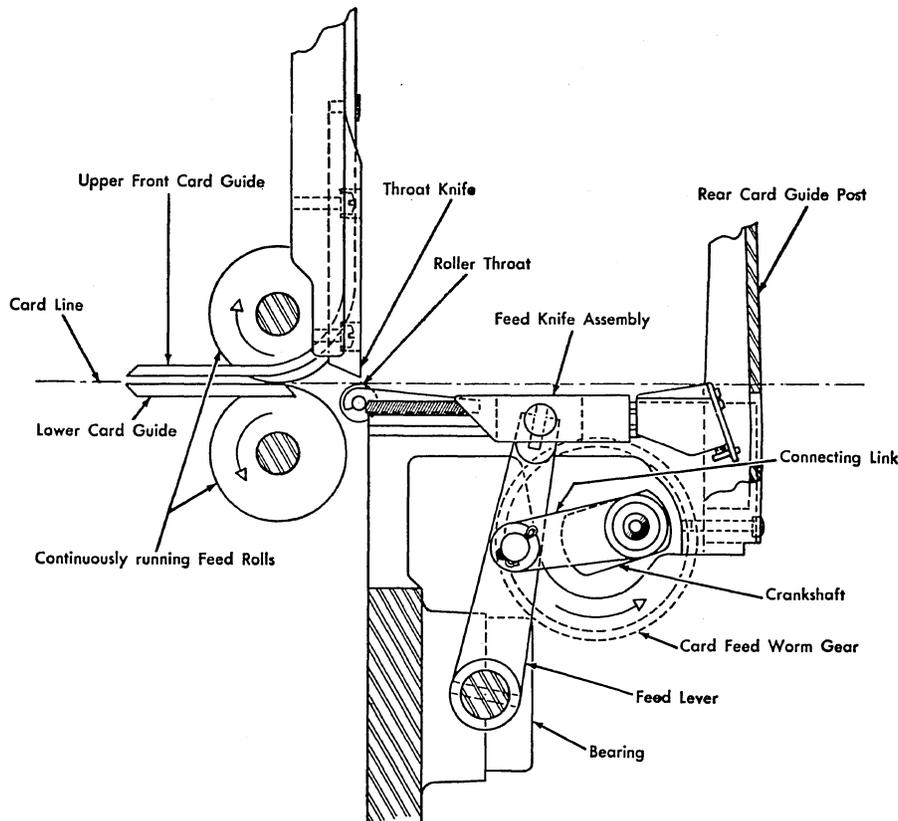
Figure 17. Feed Knife Operation
